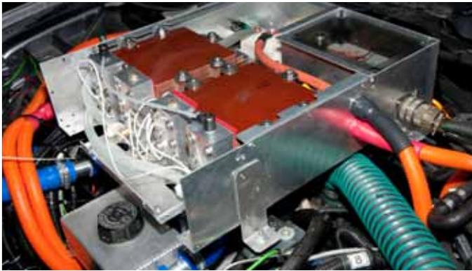
**SHOCK AND VIBRATION TESTING** with simultaneous power cycling was carried out in our own laboratories to current automotive and traction standards (spectrum to Jaguar Land Rover specification, five hours in each axis).
